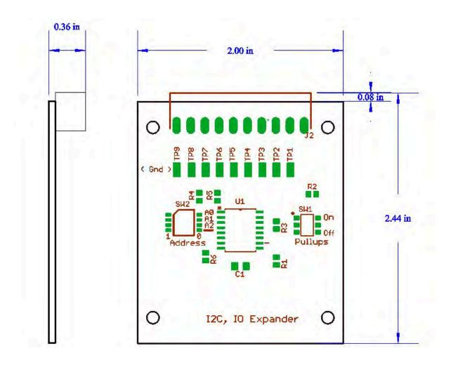
Please note: Side view only shows highest component above the module mounting surface.
